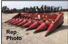
2012 3408 corn head, poly snouts, hyd deck plates, 6 spline drive shaft .....JUST IN
